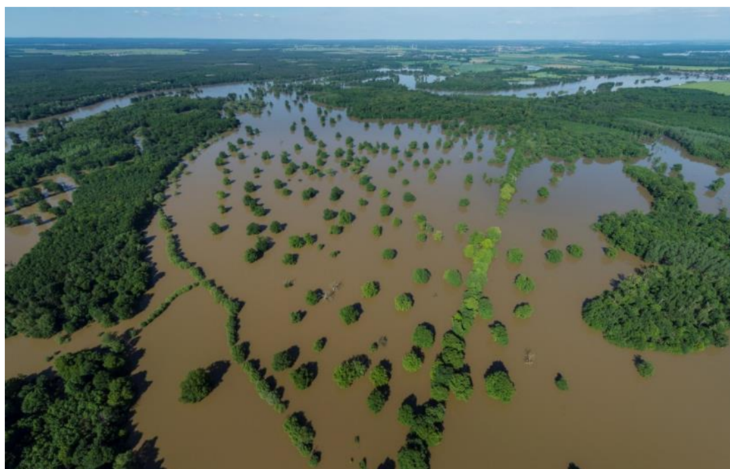
Figure 6: Floodplains reduce flood peaks by holding back floodwaters, Elbe flood, Germany, June 2013 (Source: André Künzelmann, UFZ).
