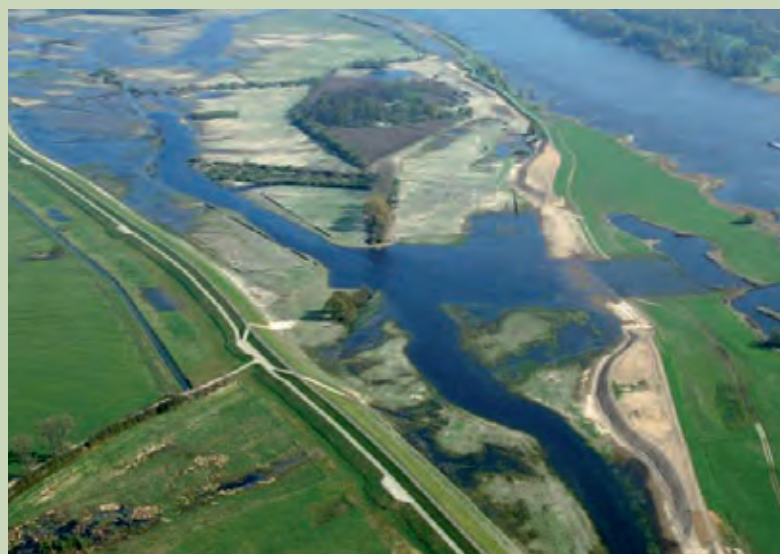
Dike relocation near Lenzen with new floodplain between old dike (right) and new dike (left)
