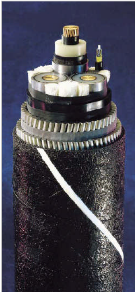
Fig. 6 Cables manufactured by Nexans Norway AS; Left: 52 kV XLPE insulated composite power and fibre optic cable employed at the Troll field in the Norwegian sector of the North Sea (AC), right: HVDC 250 kV/250 MW cable with integrated return conductor and fibre optic element (Nexans Norway AS 2005).
