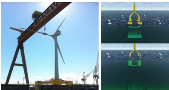
Fig. 15. Prefabrication of semisubmersible WindFloat (left, © Principle Power Inc.). TLP GICON-SOF installation concept with ballast anchor (right, © GICON).
