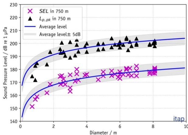
Fig. 1. Measured Peak Levels ( $L_{Peak}$ ) and broadband Sound Exposure Levels ( $SEL_{50}$ ) normalised to a distance of 750 m to the source during impact pile driving at various OWFs as a function of pile diameter (Bellmann et al. 2018).
