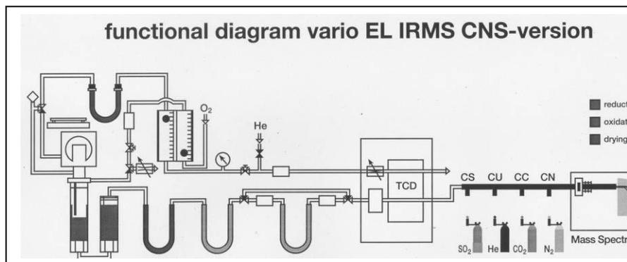
Semi-quantitative analysis of ivory was done for the elements carbon (C), nitrogen (N) and hydrogen (H) using an automatic elemental analyzer Vario EL apparatus (Elementar Analysensystem, Hanau, Germany). The working principle is shown. The principle of this method comprises three steps:
