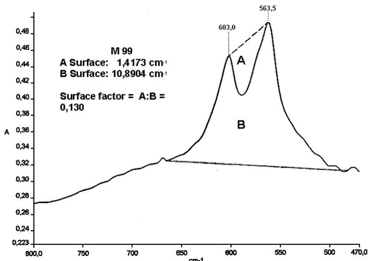
Figure 7 – FTIR Spectrum for the evaluation of the crystallinity on a well preserved sample of mammoth ivory
