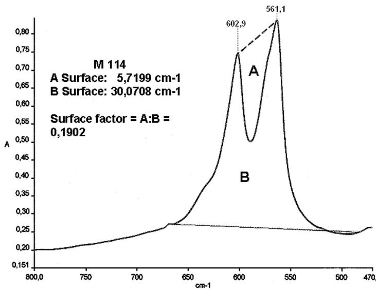
Figure 8 – FTIR Spectrum for the evaluation of the crystallinity on a very weathered sample of mammoth ivory
