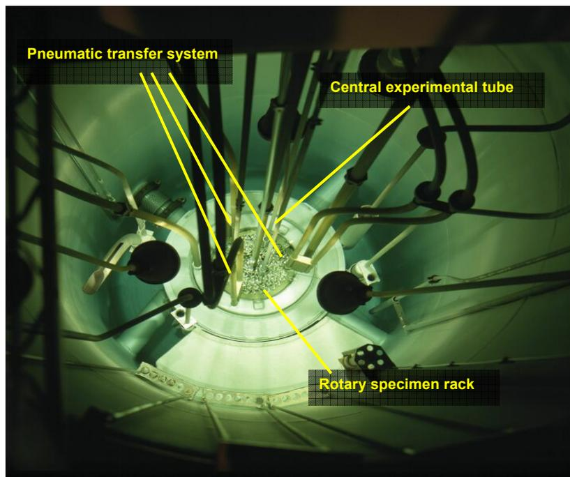
Fig. 1: Irradiation positions for the NAA at the TRIGA Mainz
