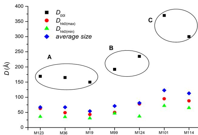
Figure 6 - Average crystallite size along  $[00l]$  and  $[hk0]$  directions
