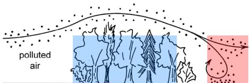
Fig. 1: Modification of airflow leads to areas with increased particle concentration (red) and decreased particle concentration (blue). After FELLEBERG (1999:41), modified
